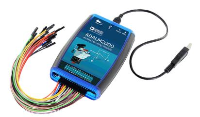
Unlike benchtop instruments, the ADALM2000 does not have a display, and it is not controlled using buttons, keys, knobs or switches. It connects to a computer through a standard USB interface, which provides both electrical power to the device, and communication and control. In addition to the USB connection, it has several input/output wires that can be used for building electronic circuits:
